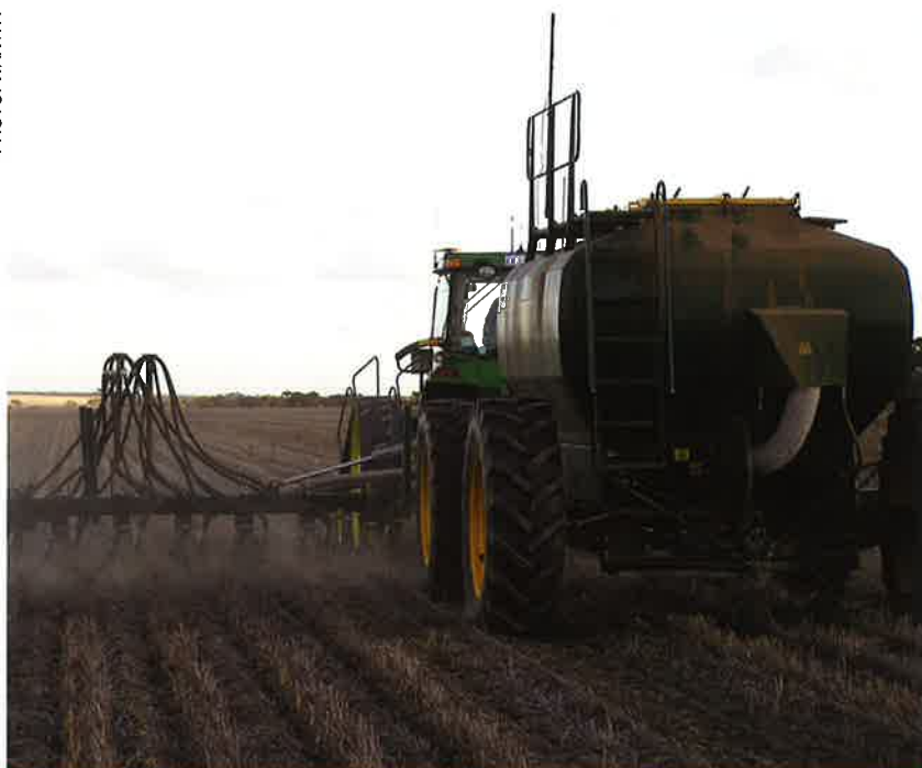
The use of discs as seeding implements or openers results in very little soil or residue disturbance so that full surface residue cover is maintained during the next crop establishment and growth.
